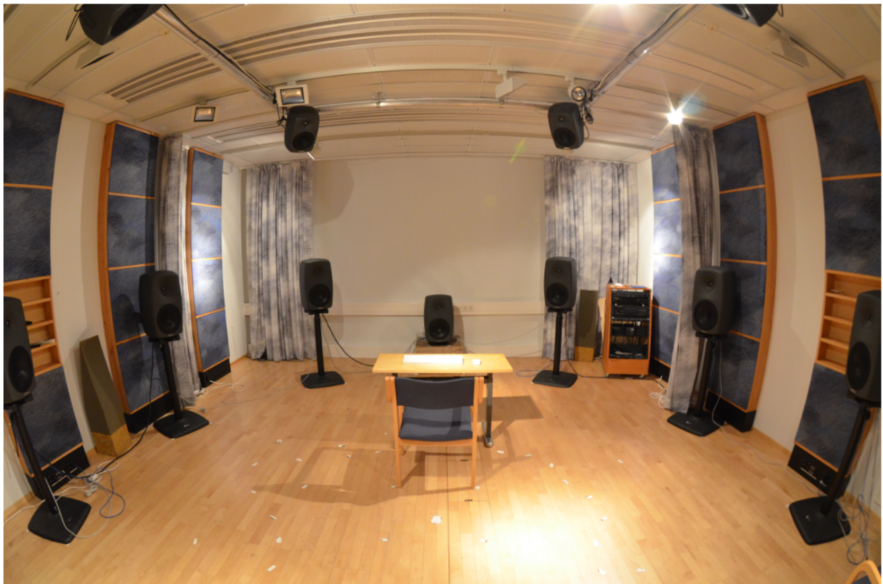
Figure 3.6a: A photograph of the listening test setup. The two rear loudspeakers at angles \pm 160^\circ are not visible in the photo. The ceiling loudspeakers were not used in the test.
